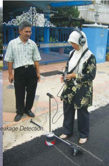
water with highly sensitive sensors (referred to as accelerometers) on the outside of the pipe wall. The usual point of contact is on the metallic valve spindle of a fully open valve.
